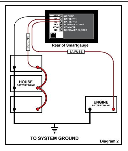
Once the ground and positive sense wires are connected, the monitor display will indicate the software and battery model revisions. The Smartgauge will then show "bt 1" in the display and the PGM/Batt 2 LED will be flashing. Use the STATUS button to scroll through the program choices, as listed below:
