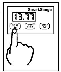
will also be displayed and will remain displayed to alert the user to a problem – until a button is pressed. If the battery voltage remains below the low-voltage warning for the set battery type an "E02" error will be displayed. If the battery voltage remains above the high-voltage warning for the set battery type, an "E03" error will be displayed.
