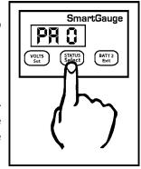
is set (using the SELECT and SET buttons) the display will again show "xx.xx" which is the upper voltage trip point.
