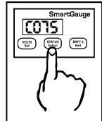
To revert to the voltage or charge status of the house battery bank, press the VOLTS button or the STATUS button.
