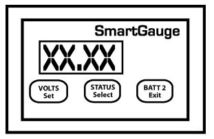
voltage will have to rise to in order to deactivate the alarm. This is the deactivation voltage. The factory default for this is 13.20 volts. Pressing the Select button will scroll this value up to 16.50 volts, it will then wrap round to whatever value was previously entered for the alarm activation voltage. This means that no matter what you do, Smartgauge will not allow this value to be set lower than the activation voltage.
